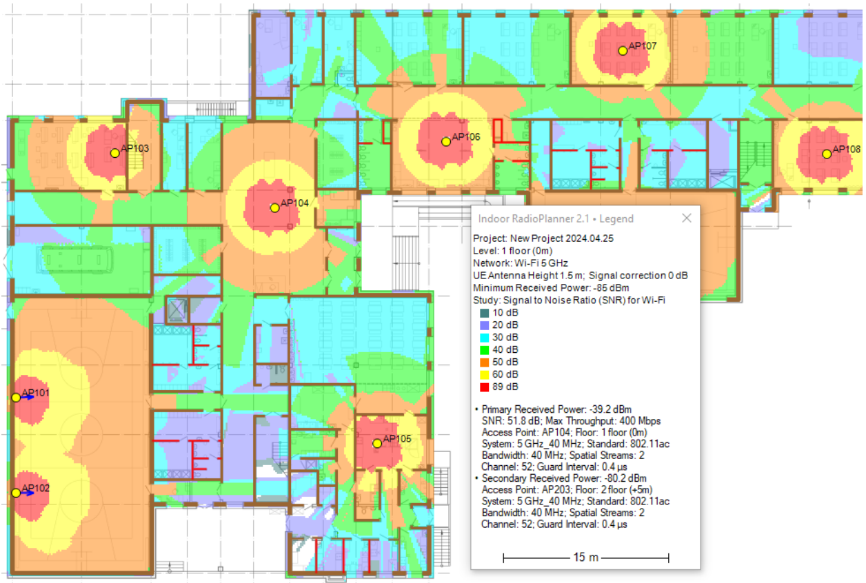
Signal to Noise Ratio (SNR) for Indoor Wi-Fi Network
