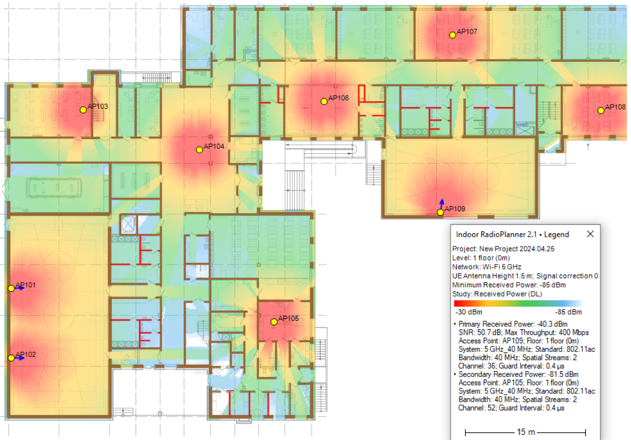
Indoor Received Power (RSSI) Coverage Prediction for Wi-Fi
