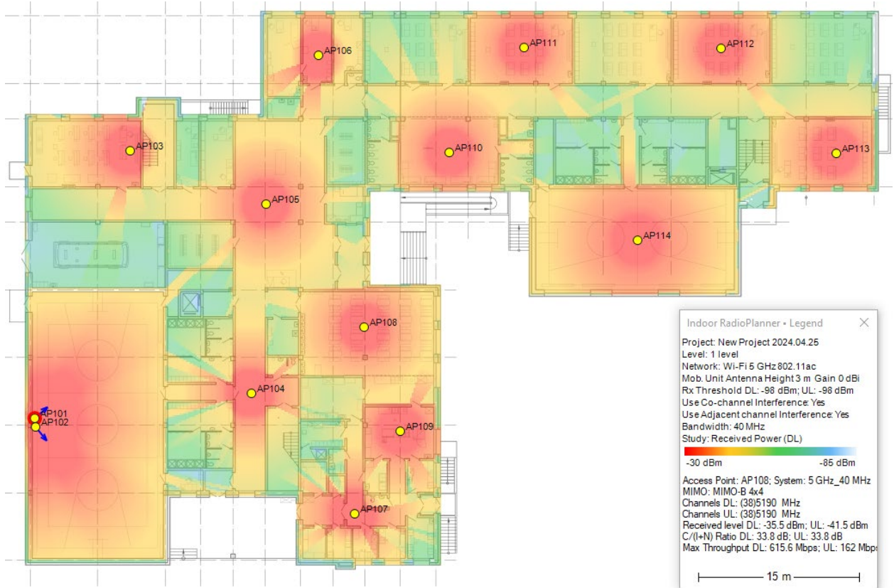
Indoor Uplink Received Power Coverage Prediction
