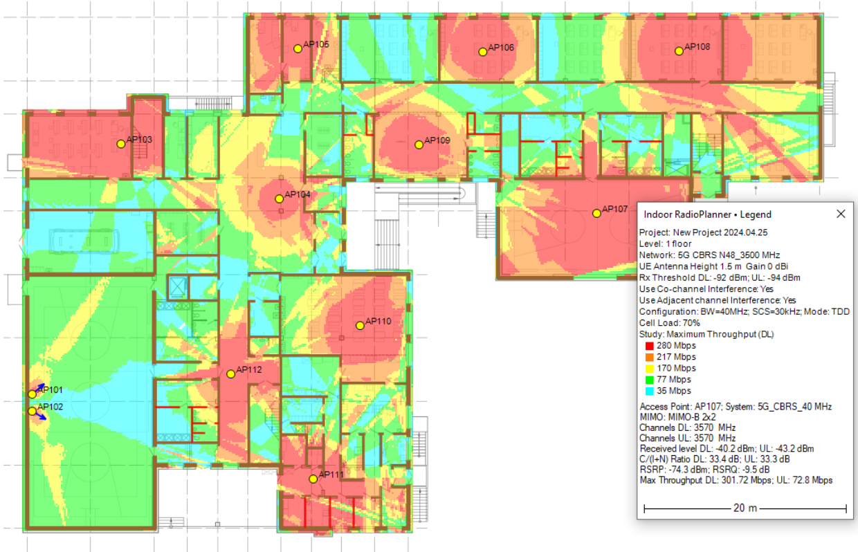
Maximum Downlink Throughput Coverage Prediction for indoor 5G CBRS N48 (3500 MHz) Network
