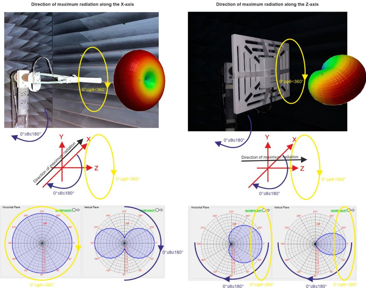
If during measurements on the stand the antenna was positioned with maximum radiation along the X-axis, then it is necessary to convert the antenna radiation pattern from 3D to 2D using the tool **Transform 3D antenna pattern with maximum radiation along the X-axis to 2D antenna pattern**.
