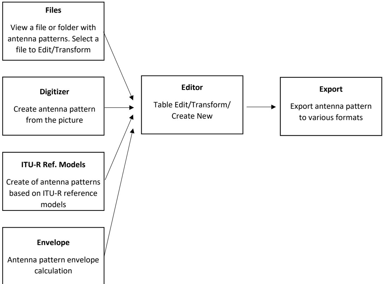
The general principle of Antenna Pattern Editor's operation can be understood from the block diagram above. The program has several blocks, each with its own function:
